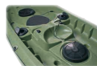
Fishing range kayaks are fitted with rod racks and watertight hatches for carrying extra equipment.
