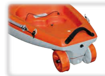
Land use configuration Wheels mounted on their axle
